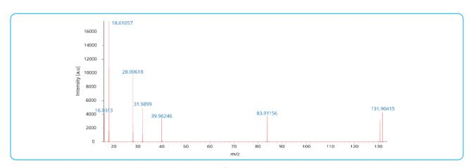
Fig. 1 Mass spectra of CH<sub>4</sub>, H<sub>2</sub>O, N<sub>2</sub>, CO, O<sub>2</sub>, Ar, Kr, Xe
