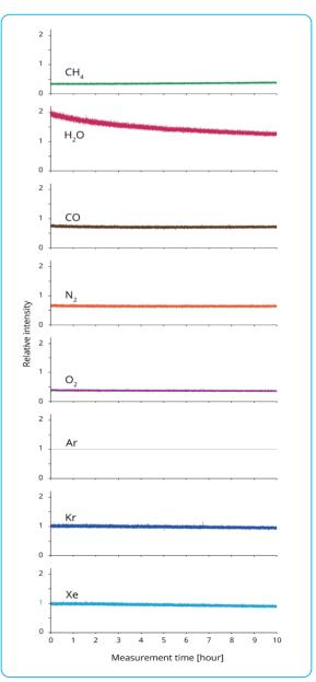
Fig. 3 Mass chromatogram of CH<sub>4</sub>, H<sub>2</sub>O, N<sub>2</sub>, CO, O<sub>2</sub>, Ar, Kr, Xe
