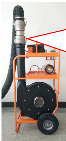
High flow Duct testing under positive pressure
