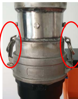
Cam lock adaptor in locked status.
