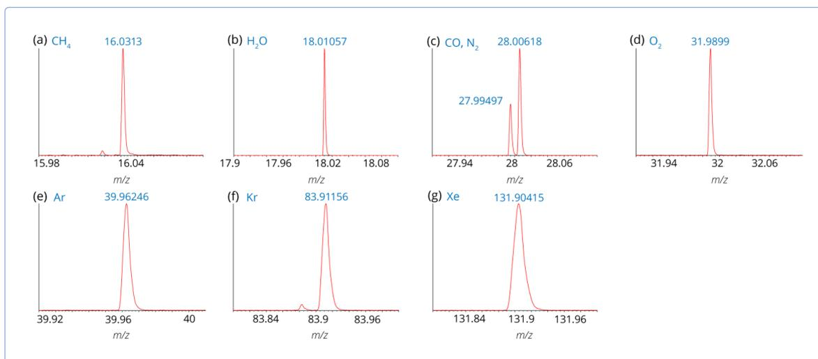
Fig. 2 Mass spectra of CH<sub>4</sub>, H<sub>2</sub>O, N<sub>2</sub>, CO, O<sub>2</sub>, Ar, Kr, Xe (enlarged near peak regions)
