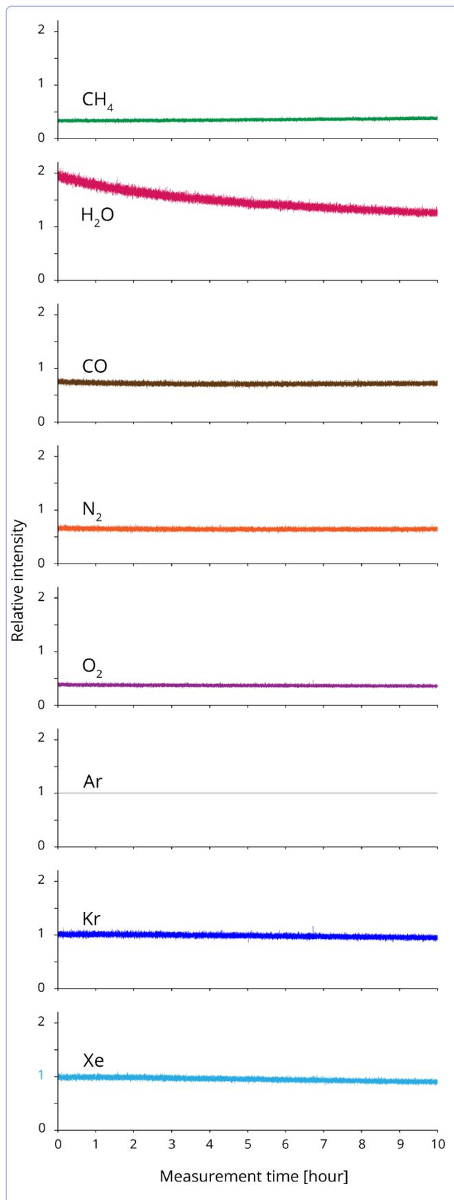
Fig. 3 Mass chromatogram of CH<sub>4</sub>, H<sub>2</sub>O, N<sub>2</sub>, CO, O<sub>2</sub>, Ar, Kr, Xe
